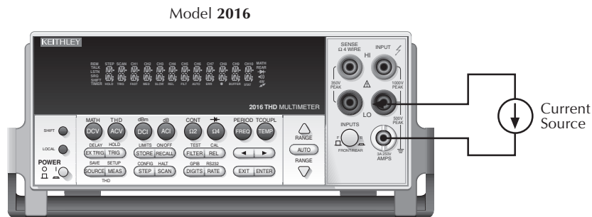
Figure 2-5 DC and AC current measurements
